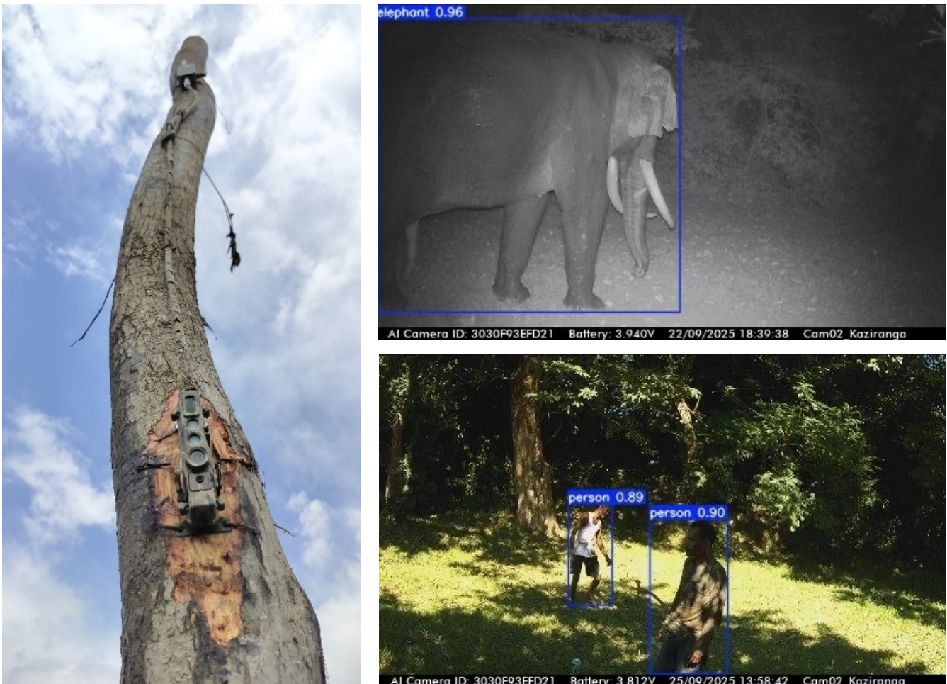
Figure 52: Setup of AI Trail Guard Camera showing identified picture of elephant (top right) and humans (bottom right)
