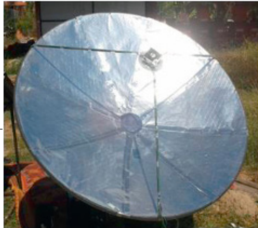
Solar parabolic concentrator coupled to TE module and Fan Orientation 39
